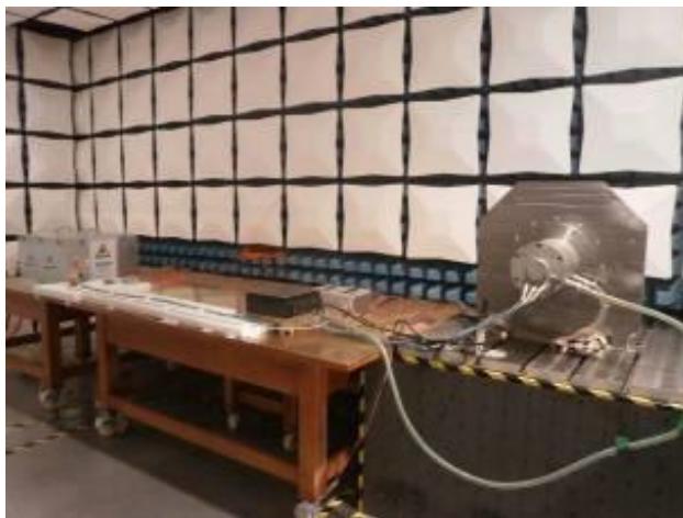
Fig. 5. Test setup for conducted emission
